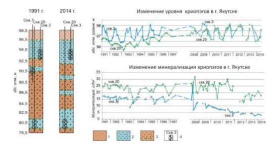
Fig. 3. Logs showing the position of cryopeg layers and curves demonstrating the dynamics of cryopeg levels and dissolved-solids content.
