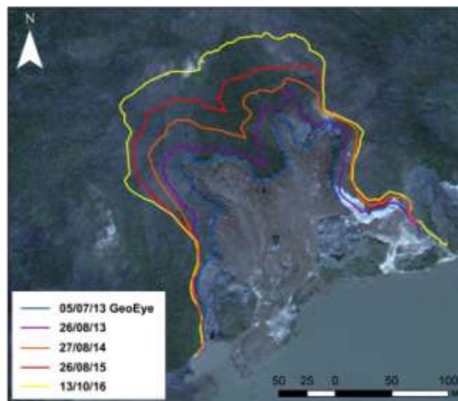
Fig.3. Retreat of the edge of the thermo-cirque with massive ice bedding at the Central Yamal. Cartography background: space image GeoEye-1 dated 05.07.2013 y. (Digital Globe Foundation)
